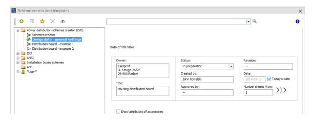
Scheme creator allows user to select products available in the modular apparatus library and place them in specific positions in the scheme. We will start our work by inserting a 3P switch disconnector
