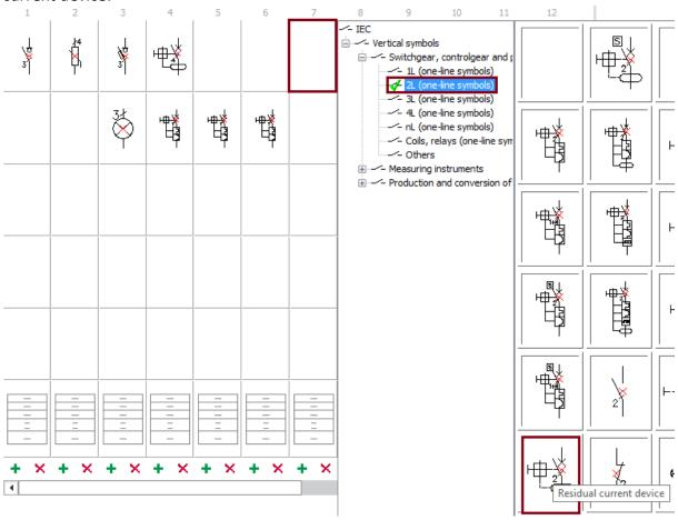
Afterwards we will insert a 1P modular circuit breaker into the diagram just below the RCD. This time, we will choose the *CLS6-B10* product previously prepared by us as the type.
