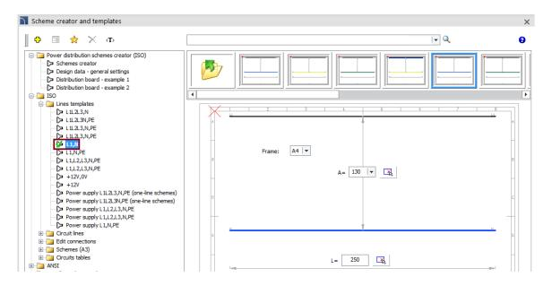
We select the frame as A4 and dimension A as 130. Dimension L (i.e. the width of the potential line) we will determine directly from the drawing. To do this, we click the button and then we define the L dimension by indicating two consecutive points P1 and P2.
